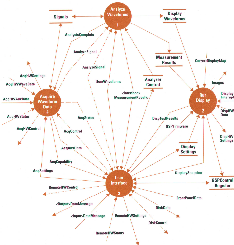
Fig. 1. Top-level data flow diagram for the HP 54720/10.
